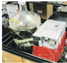
Example RSSCT set-up. Photo courtesy of Dr. Knappe, NCSU.
